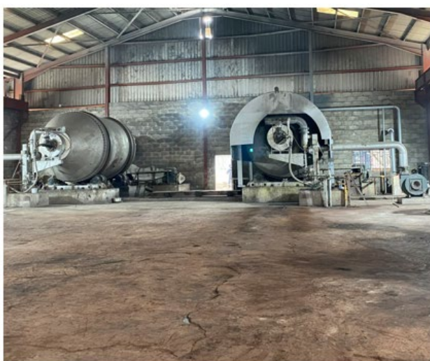
Main smelting hall with the two installed rotary furnaces
