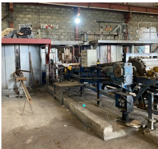
Refining kettles with automated casting machine
