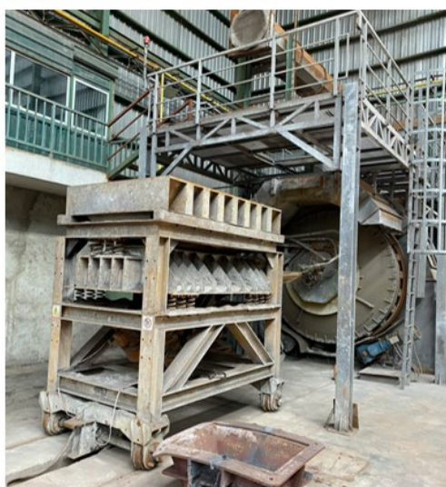
Housed-in rotary furnace with automated charger (meanwhile replaced by a more modern furnace)
