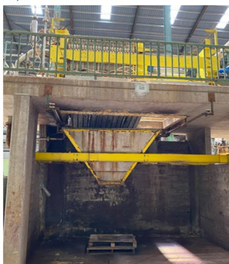
Filter press to reduce the moisture content of desulfurised battery paste (desulfurisation prior to smelting)
